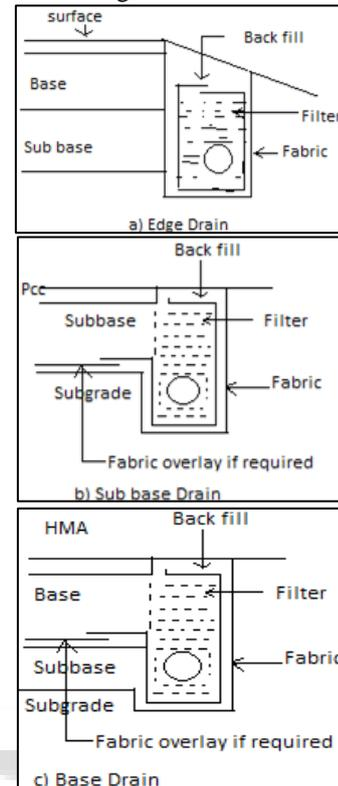
Fig. 2: Application of Geo Textile
