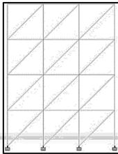
Fig. 2: Open ground storey building with all storey infill strut wall (proposed model)
