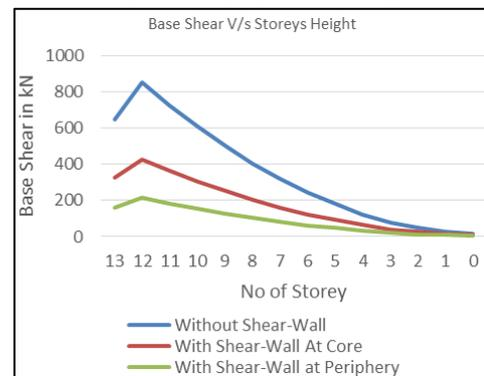
Fig. 6: Base Shear Values V/s Storeys Height.
