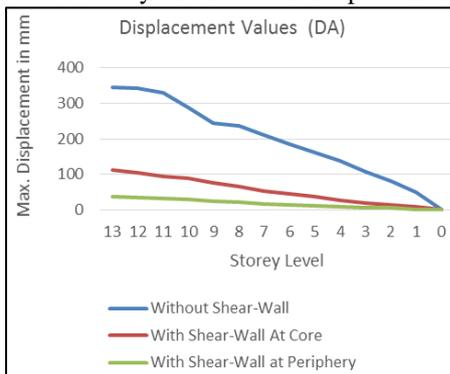
Fig. 8: Maximum Displacement V/s Storeys Height.
