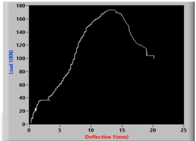
Fig. 7: Load Vs Deflection for Bubble Deck Slab of 70mm Dia Voids
