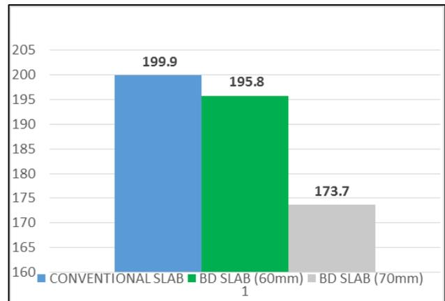
Fig. 8: Graphs for the comparison of ultimate loads of the three slabs
