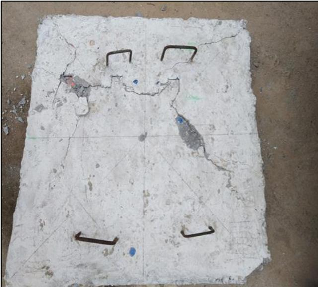
Fig. 9: Cracks developed in the slabs after failure
