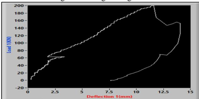
Fig. 5: Load Vs Deflection for Conventional Slab
