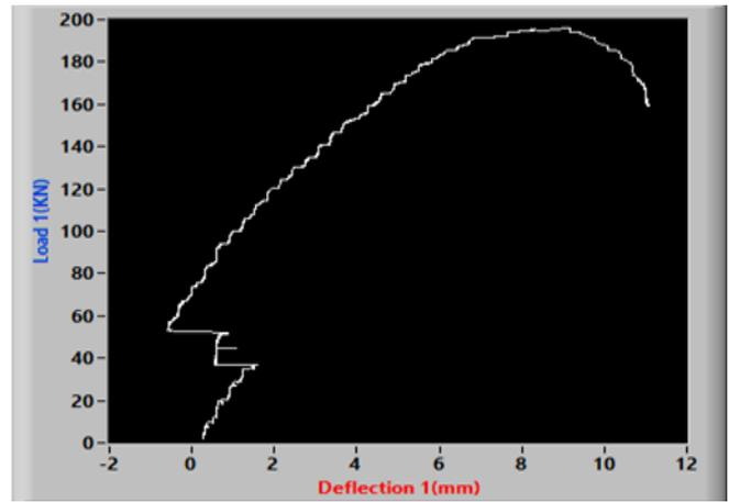
Fig. 6: Load Vs Deflection for Bubble Deck Slab of 60mm Dia Voids
