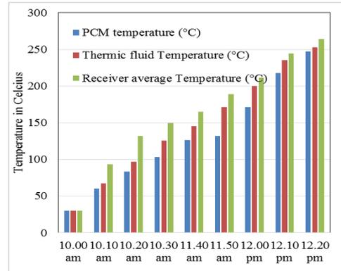
Fig. 4: Temperature trend of sensible and latent heat materials (26<sup>th</sup> April 2017)
