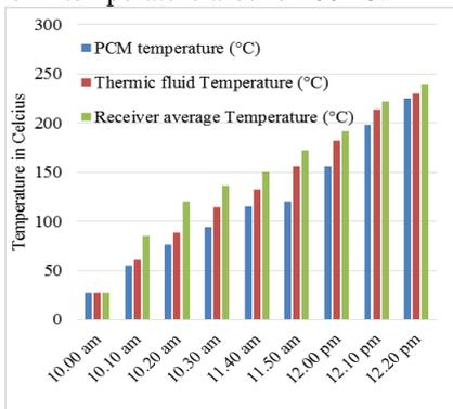
Fig. 3: Temperature trend of sensible and latent heat materials (25<sup>th</sup> April 2017)
