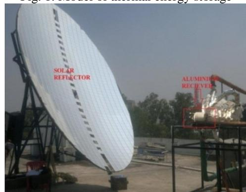
Fig. 2: Concentrated solar collector
