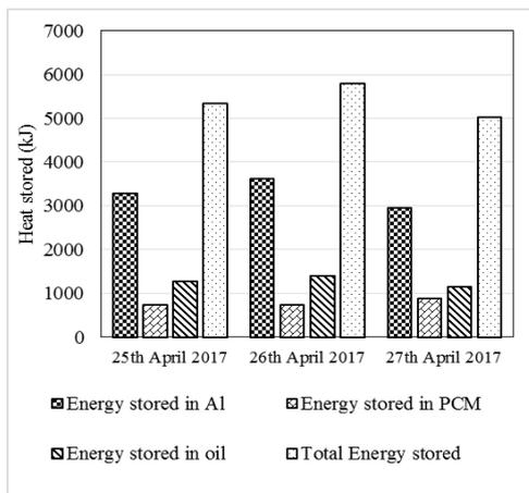
Fig. 7: Energy stored in the solar receiver
