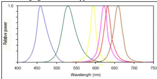
Fig. 2: Spectral power distributions of several types of LEDs
