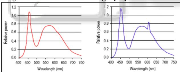
Fig. 3: Spectral power distributions of early phosphor-based white LEDs (left), and white LEDs using more recently developed phosphors (right) with increased output between 600 and 650 nanometers.
