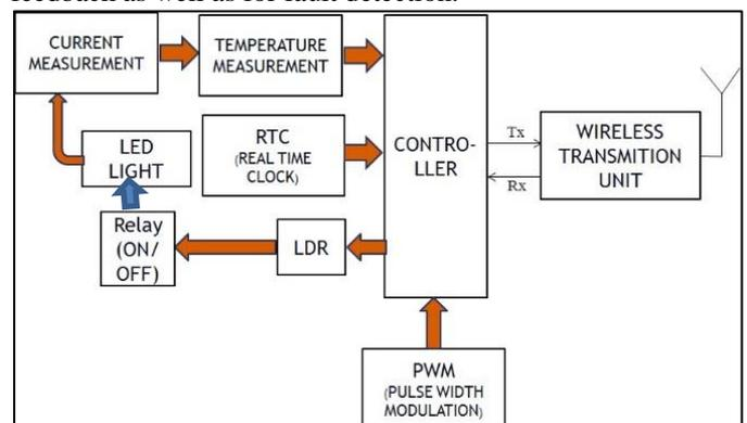
Fig. 6: Systematic block diagram of sensor node
