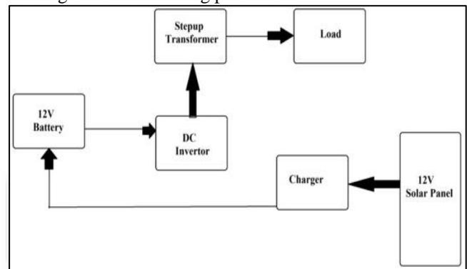
Fig. 1: Solar Inverter Schematic
