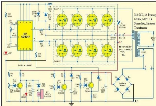
Fig. 2: Inverter circuit [courtesy of <http://electronicsforu.com>]
