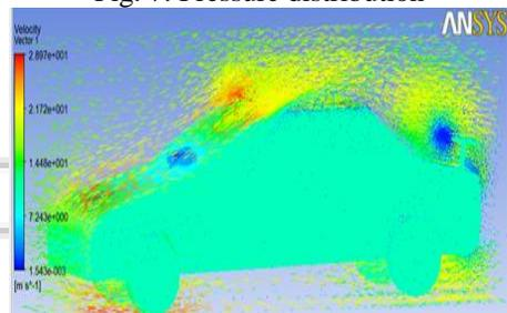
Fig. 8: Vector plot of velocity
