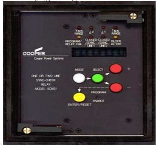
Fig. 1: Front View of the SCM21 Synch-Check Relay
