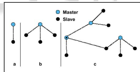
Fig. 1.3: Topologies: Piconets with single slave operation (a), multi-slave operation (b) and scatternet operation (c).
