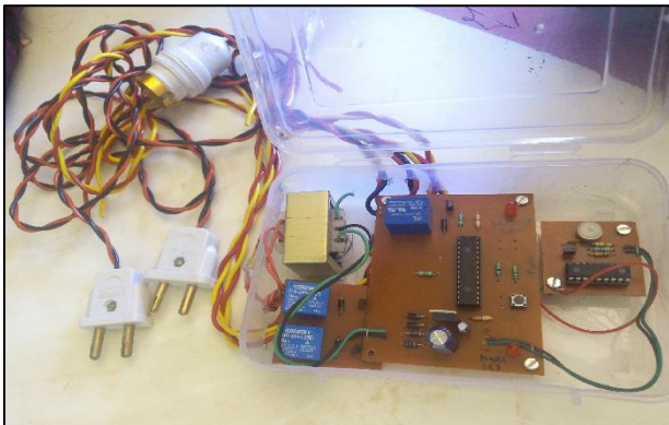
Fig. 6: Circuit is in off condition when user claps then device will be ON.
