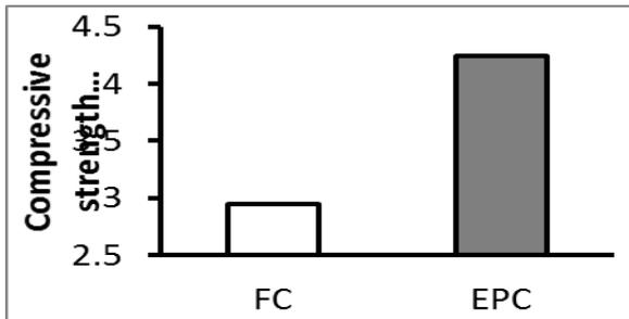
Fig. 4: graph showing compressive strength of the cubes
