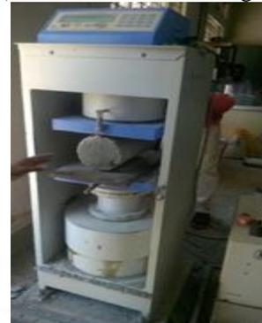
Fig. 2: Split Tensile Strength in the Testing Machine
