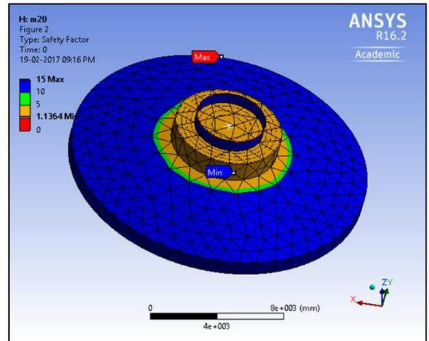
Fig. 5: Safety Factor Of The Model
