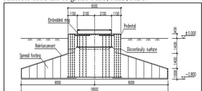
Fig. 1: Cross section of the foundation.
