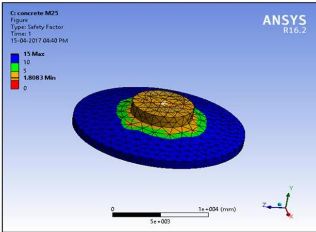
Fig. 8: Safety Factor Of Model
