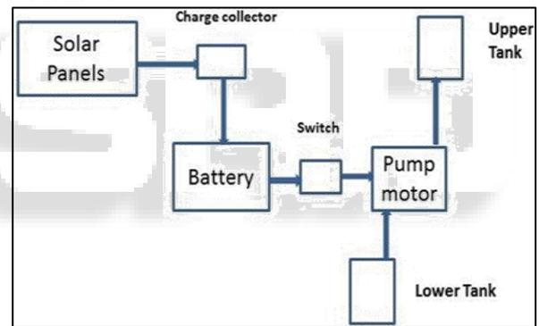
Fig. 1: (Proposed Diagram of Solar Water Pumping System for Domestic Purpose.)
