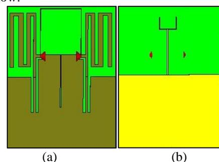
Fig. 1: Initial antenna design without defects and stubs. a) Front view. b) Back view.
