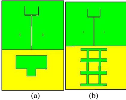
Fig. (2): Ground plane a) with T-shaped DGS. b) With EBG inspired DGS with gap=0.
