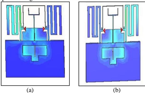
Fig. (6): Current Distribution (a) When antenna 1 is excited (b) When antenna 2 is excited.
