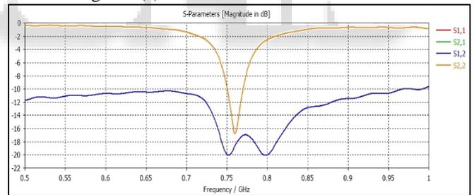
Fig. 5(a): simulation results with T-shaped DGS.
