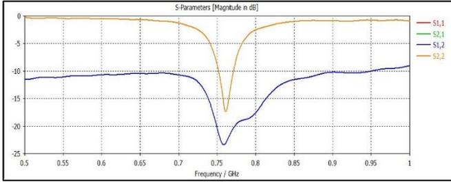
Fig. 5(c): Simulation results with stub lines and T-shaped DGS.
