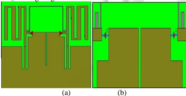
Fig. (3): (a) Model with stubs (b) Focussed view of the location of the stubs.
