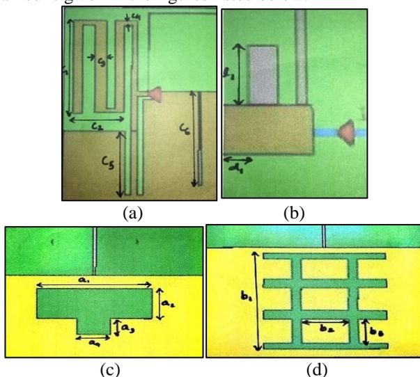
Fig. 4: Design specifications of a)Antenna b) Stub line C) T-shaped DGS d) EBG inspired DGS.
