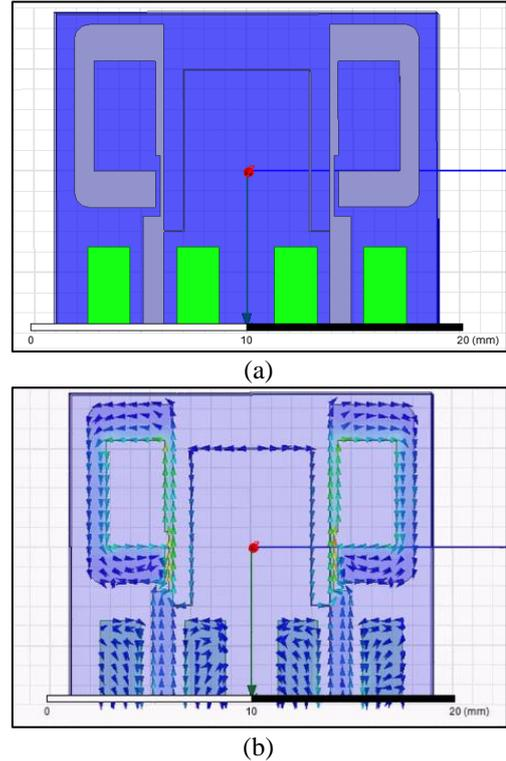
Fig. 4. Design of Antenna (a) with Neutralization Line (b) Surface Current Density
