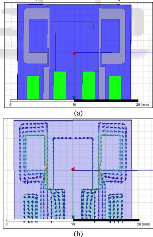
Fig. 5: Design of Antenna (a) with Neutralization Line and Extended Ground (b) Surface Current Density
