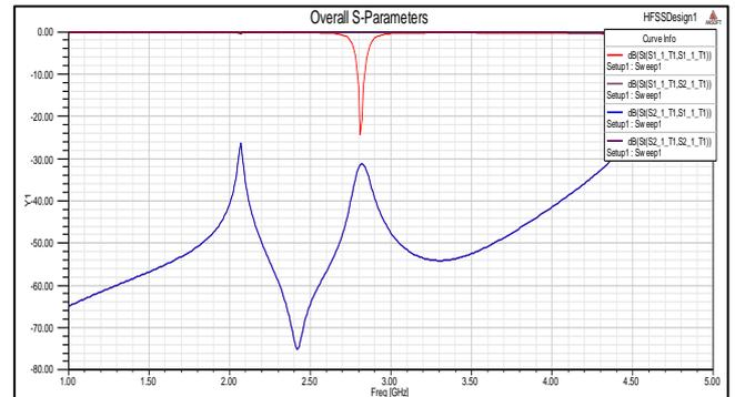
Fig. 7: Simulation Graph of the design with Neutralization Line (NL) and Extended Ground structure
