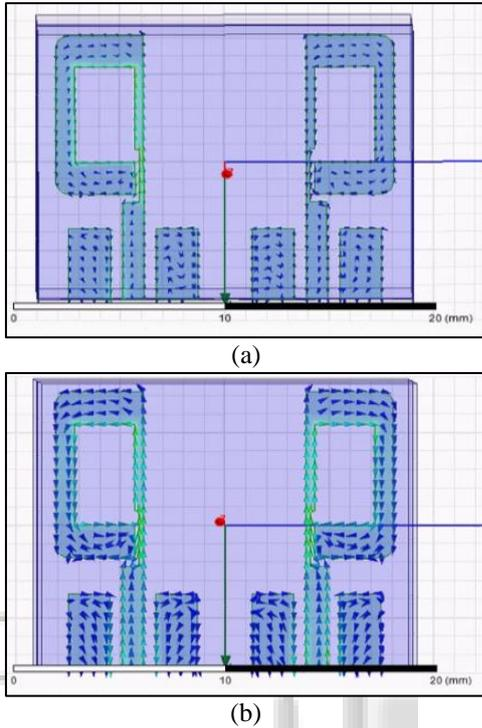
Fig. 3: Surface Current Density with (a) Single Port Excitation (b) Dual Port Excitation
