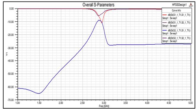
Fig. 5: Simulation Graph of the design without any decoupling structure
