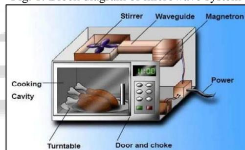
Fig. 2: Internal structure of microwave oven
