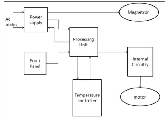
Fig. 1: Block diagram of microwave system
