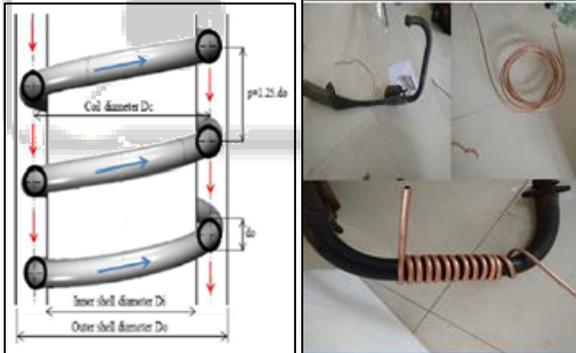
Fig. 3: Coil type heat exchanger
