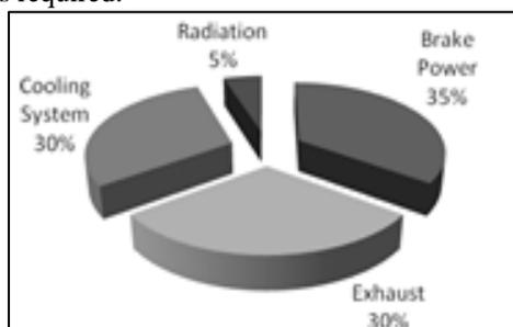
Fig. 1: Heat losses from I. C. Engine
