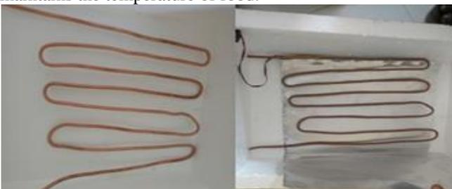
Fig. 4: Heat exchanger in Delivery box
