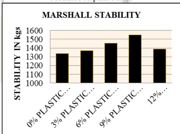
Fig. 7: Marshall Stability Values for conventional and Polycarbonate Modified Asphalt Mixes
