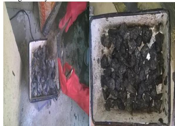
Fig. 4: Preparation of Plastic Coated Aggregates
