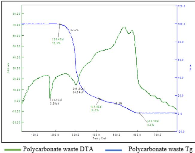
Fig. 5: Thermal Analysis Graph
