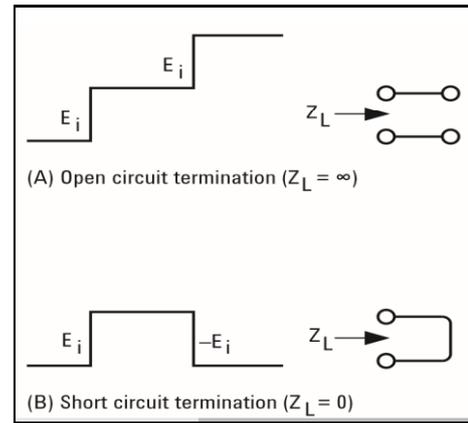
Fig. 3: Open and short circuit termination.
