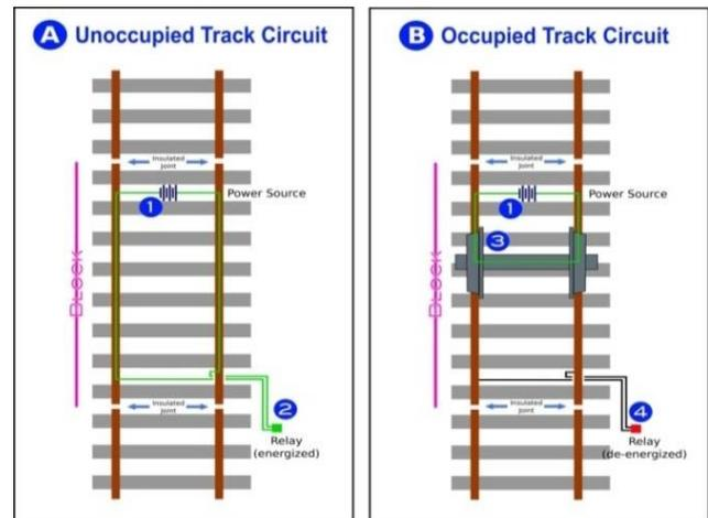
Fig. 1: Unoccupied and occupied track circuit.
