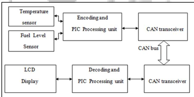
Fig. 3: Block Diagram of Proposed Work
