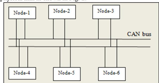
Fig. 2: Structure of Controller Area Network
