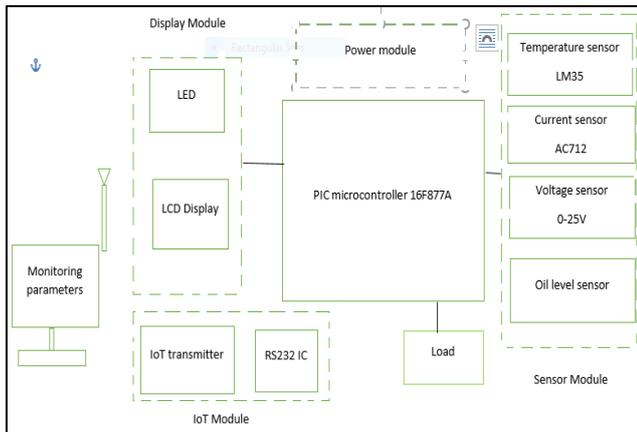
Fig. 4: Block Diagram of Circuit
