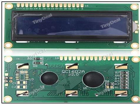
Fig. 10: LCD Display
