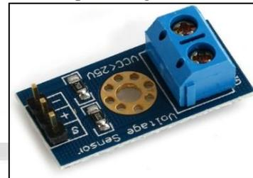
Fig. 8: Voltage Sensor
