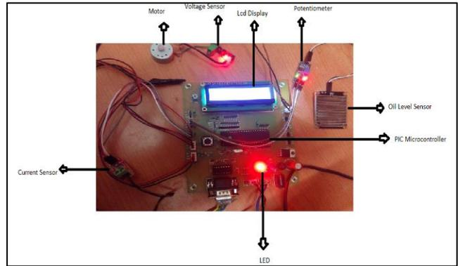
Fig. 13: Circuit Assembling
