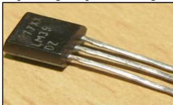
Fig. 6: Temperature Sensor
