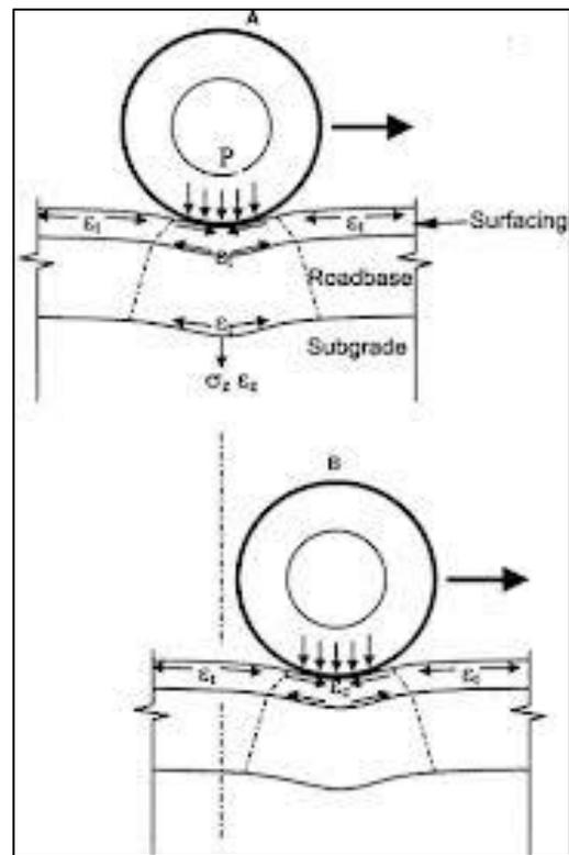
Fig. 1: Critical Locations in Pavement
