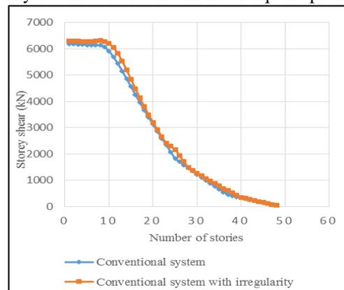
Fig. 7: Storey shear for conventional system
