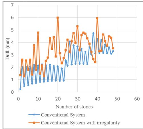
Fig. 5: Storey drift for conventional system
