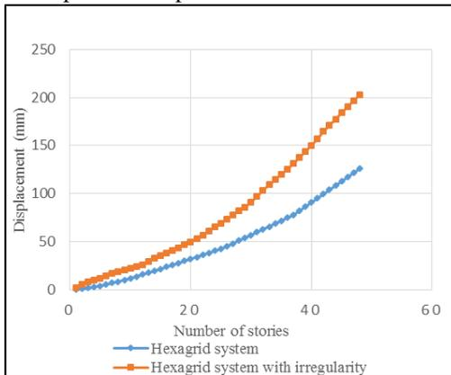
Fig. 4: Comparative displacement for hexagrid system
