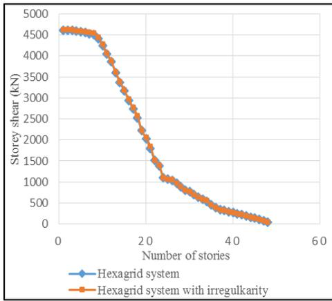
Fig. 8: Storey shear for hexagrid system
