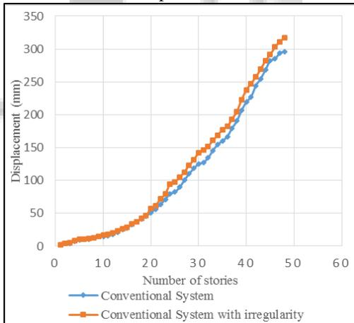
Fig. 3: Comparative displacement for conventional system
