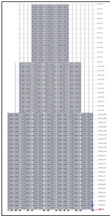
Fig. 2: Elevation of Hexagrid Building Frame
