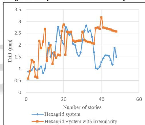
Fig. 6: Storey drift for hexagrid system
