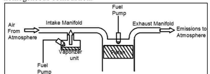
Fig. 1: Fuel Vaporizer System
