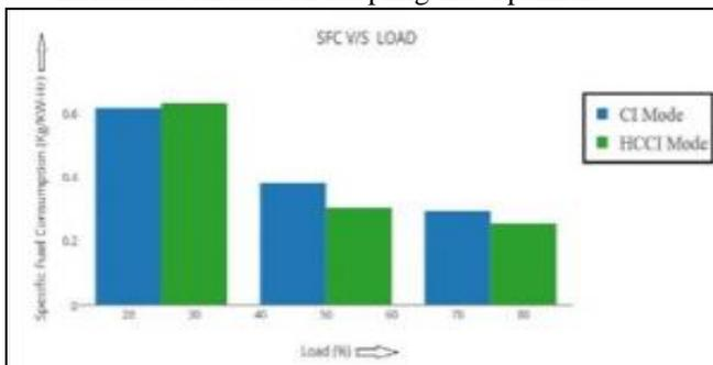
Fig. 7: SFC vs load
