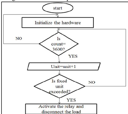
Fig. 8: Flow chart for power exceed the limit
