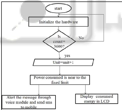
Fig. 7: Flow chart for power reach the limit
