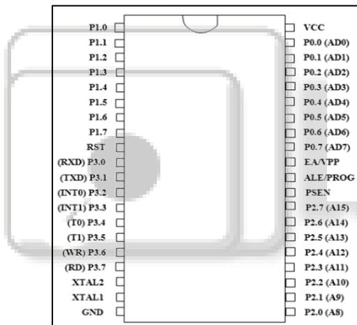
Fig. 3: Pin Diagram of 89c51 microcontroller
