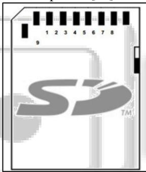
Fig. 5: SD card pin out
