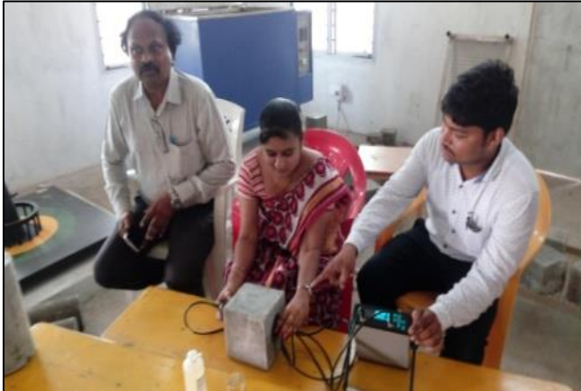
Fig. 1: UPV Cube Testing
