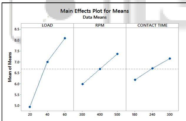
Fig. 6: Main Effect Plots for Aluminium Friction Force
