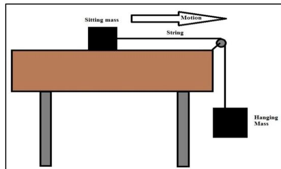
Fig. 2: Simple Tribometer principle [6]
