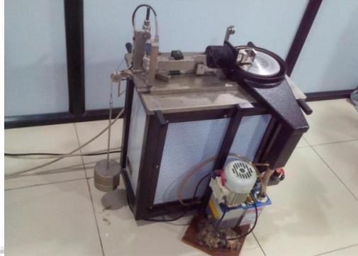
Fig. 3: Pin on Disc (DUCOM/TR-20LE-PHM-200)
