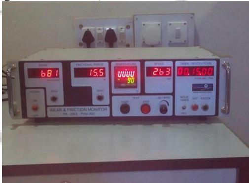
Fig. 4: Display Monitor of Frictional Force, Wear, Temperature, Speed and Timer
