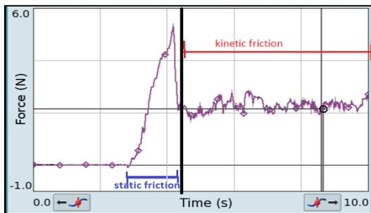
Fig. 1: Static friction and kinetic friction comparison [2]
