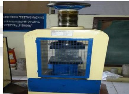
Fig. 6.1: Compression test
