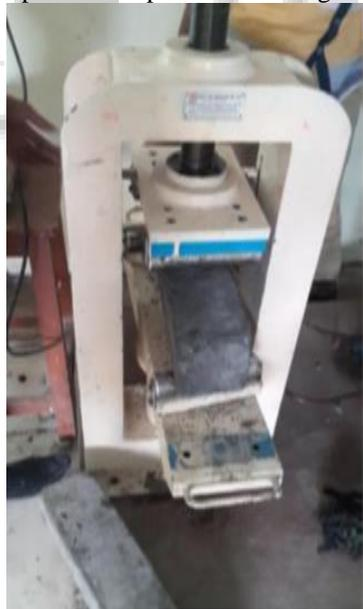
Fig. 6.5: Flexural Strength Test
