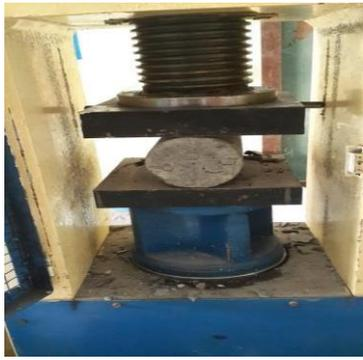
Fig. 6.3: Split Tensile Test
