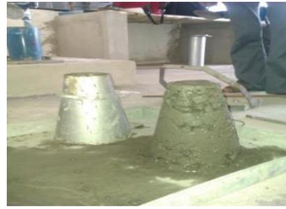
Fig. 6.1: Slump Cone Test
