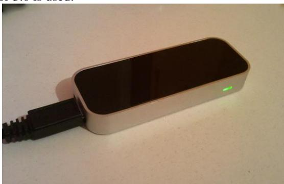
Fig. 2: Leap Motion controller with Micro-USB plug
