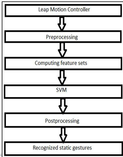
Fig. 2: System Architecture
