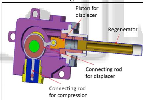
Fig. 5: Cross section of Stirling cryocooler
