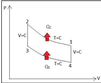
Fig. 1: P-V diagram of stirling cryocooler
