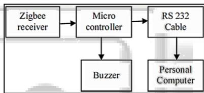
Fig. 3 Receiver Module Block Diagram
