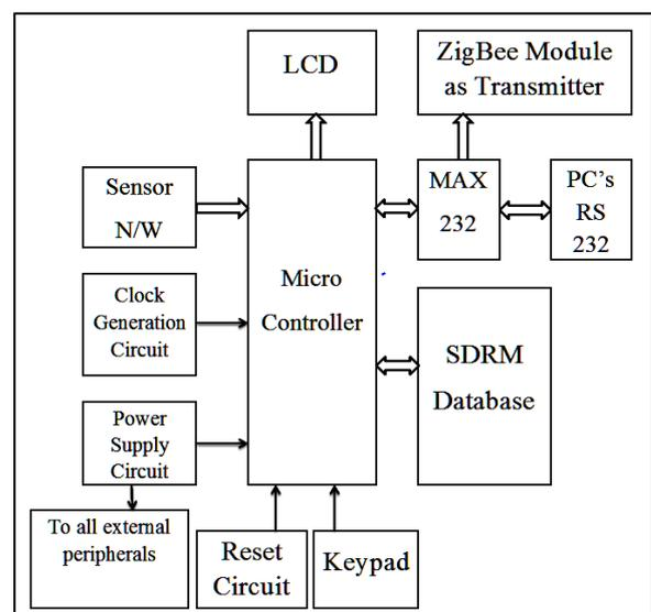
Fig. 2: Transmitter Module Block Diagram
