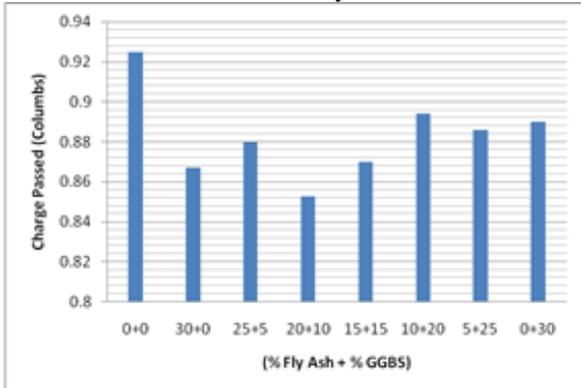
Fig. 7: RCPT after 28 Days in Different Mix
