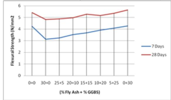
Fig. 4: Line chart of Flexural Strength of 7 & 28 days
