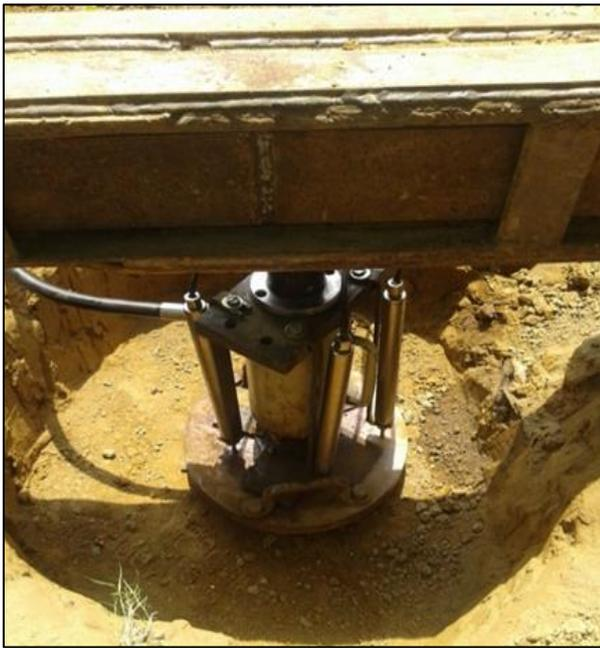
Fig. 1: Test setup of pile loading
