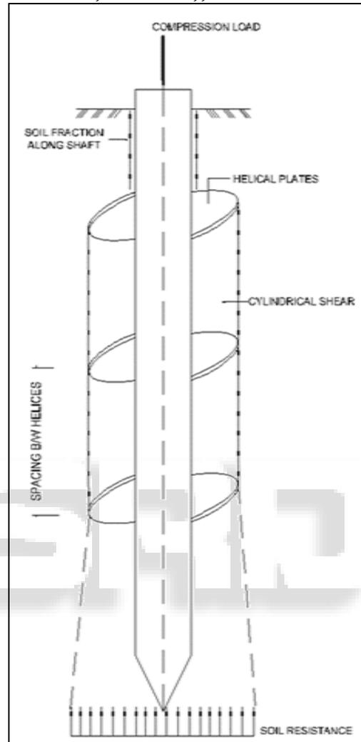
Fig. 2: schematic of a typical helical pile foundation section
