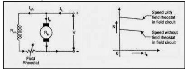
Fig. 4: Flux Control Method
