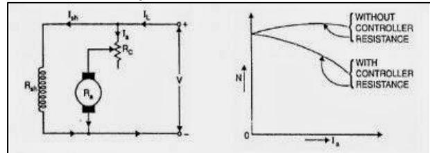
Fig. 5: Armature voltage control method
