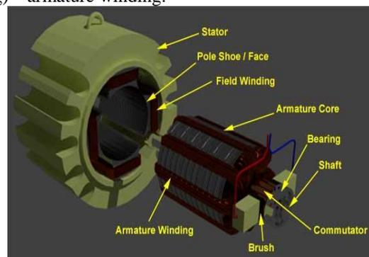
Fig. 2: Construction of Dc Motor
