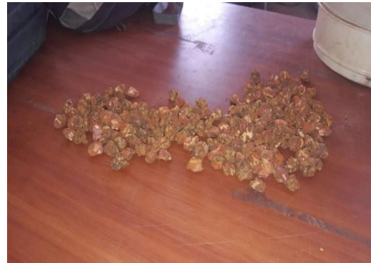
Fig. 2: 20mm laterite coarse aggregate.
