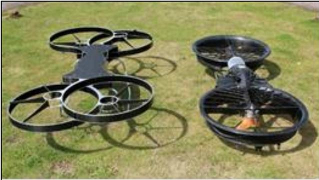
Fig. 3: Hover bike with overlapping propeller [9]
