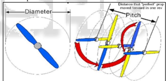
Fig. 4: Pitch of propeller [7]
