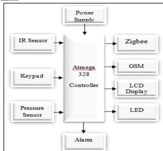
Fig. 1: Transmitter block
