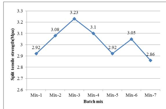
Fig. 5: Test result for Split tensile test on cylinders at 28 days (in N/mm<sup>2</sup>)
