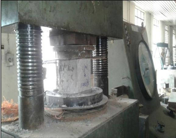
Fig. 3: Compression test on cubes
