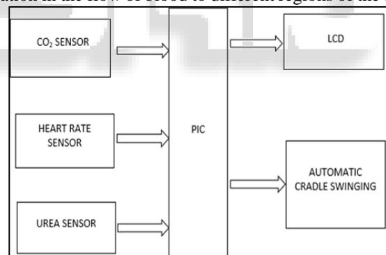
Fig 1: Block diagram of Infant Monitoring and Automatic cradle swinging system
