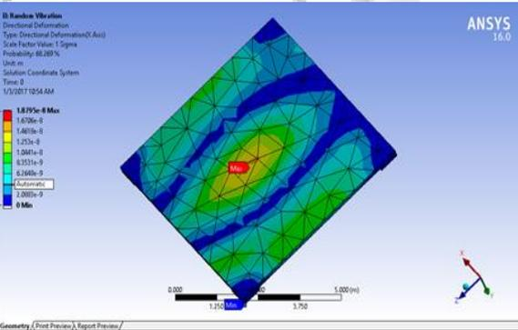
Fig. 3.7: Deformation of Flat slab Model without epoxy material
