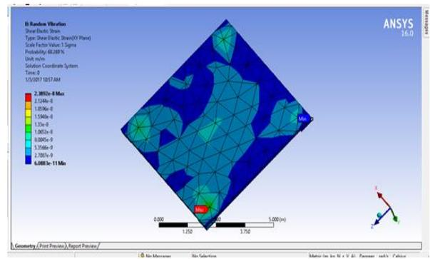
Fig. 3.9: Shear Strain of Flat slab Model without epoxy material
