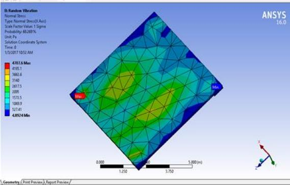
Fig. 3.6: Normal Stress of Flat Slab Model without epoxy material
