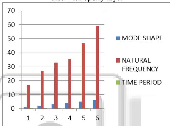
Graph. 2: of natural frequency vs mode shape for flat slab with epoxy layer
