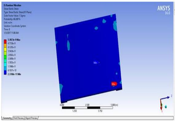
Fig. 3.5: Shear Strain of Flat slab Model with epoxy material
