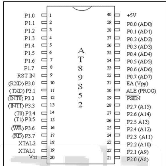
Fig. 1: Pin diagram of AT89S52 microcontroller
