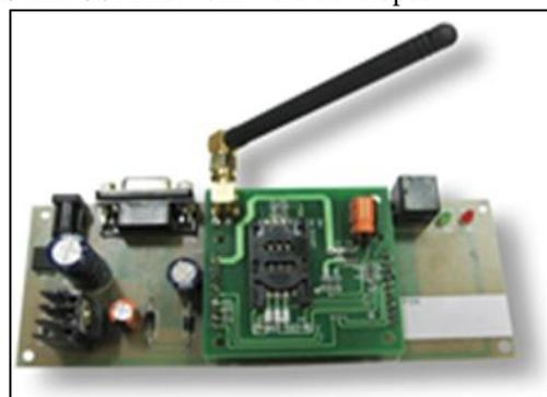
Fig. 3: GSM Modem
