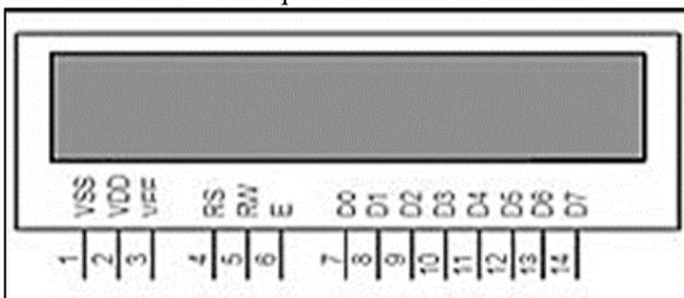
Fig. 2: Schematic diagram of LCD
