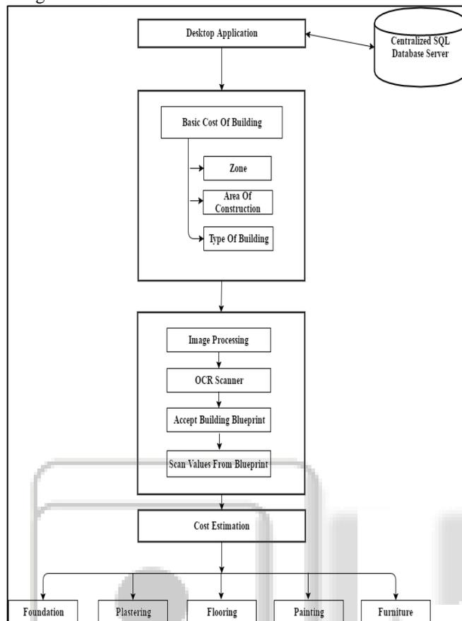
Fig. 2: Flowchart Construction Cost Estimator using Image Processing
