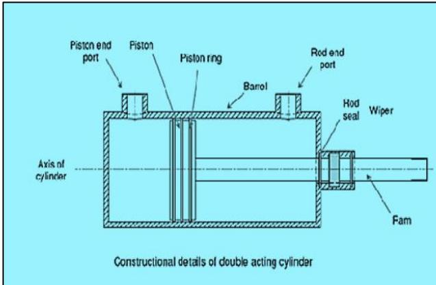
Fig. 3: Constructional details of double acting cylinder
