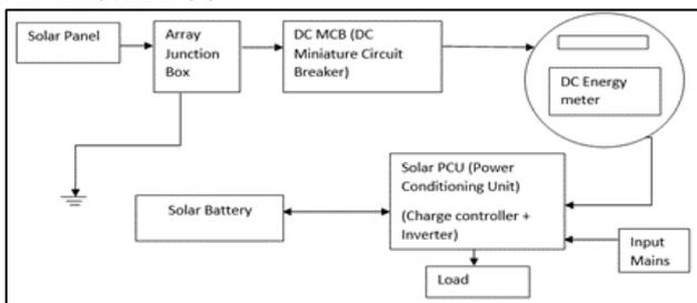
Fig. 5: Block diagram of stand-alone solar PV power generation system
