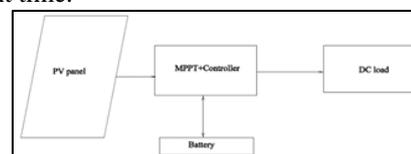
Fig. 3: Regulated stand-alone system with battery and DC load
