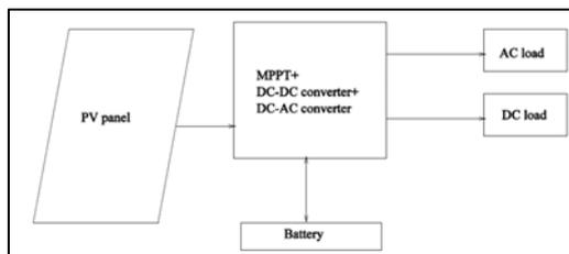
Fig. 4: Regulated stand-alone system with battery and AC/DC load
