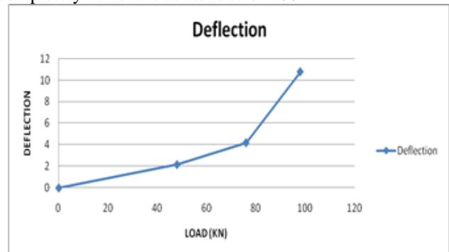
Fig. 4.2: Load versus Deflection Curve for SB1
