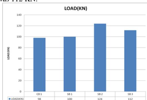
Fig. 4.5: Load comparison of various strengthened beams
