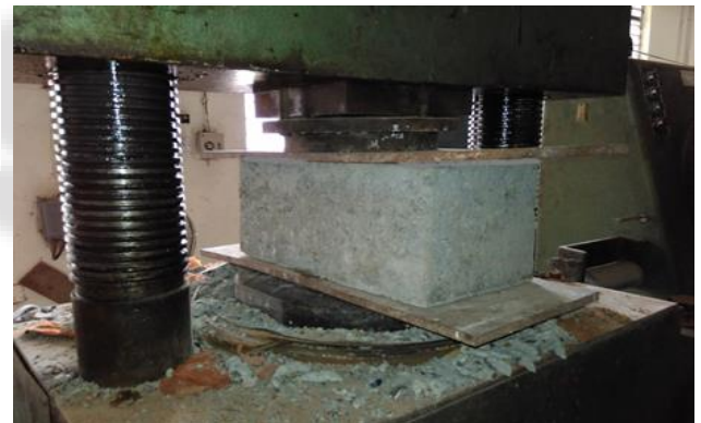
Fig. 8: Compressive Strength test for Hollow Concrete Block
