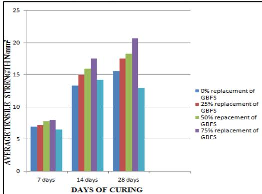
Fig. 3: Average split tensile strength on concrete
