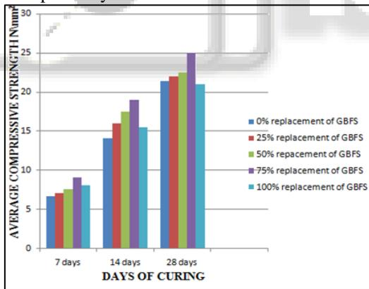
Fig. 2: Average compressive strength on concrete
