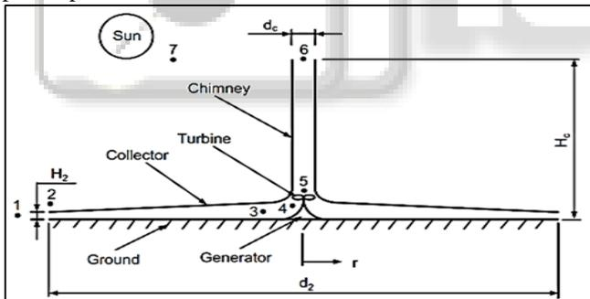
Fig. 1: Schematic illustration of a solar tower power plant
